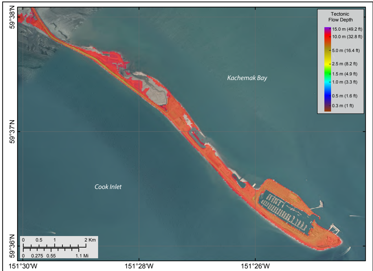
Figure 27. Modeled maximum composite flow depth over dry land for all tectonic scenarios for Homer Spit.
