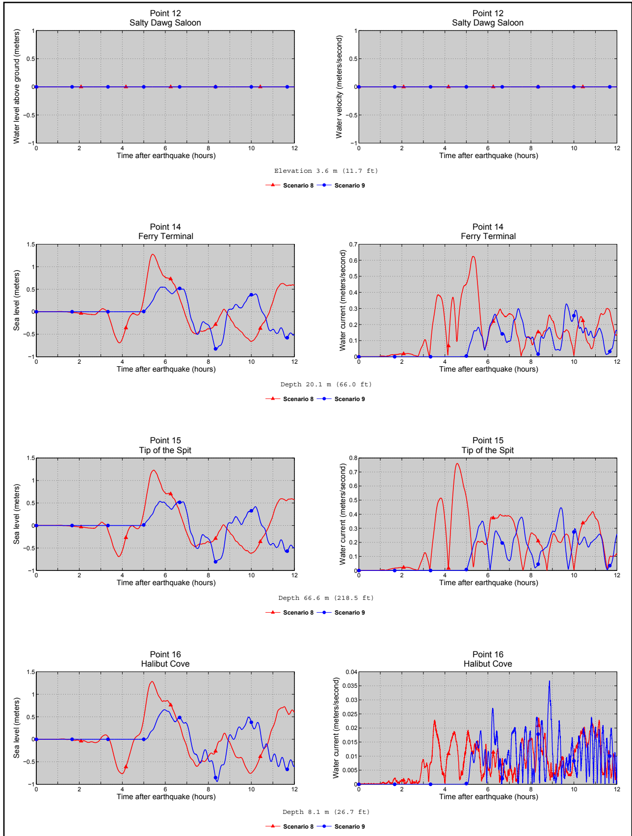
Figure A5, continued. Time series of water level (left column) and velocity (right column) for tectonic scenarios 8-9 at selected locations shown in figures A1 and A2. Elevations of onshore locations and ocean depth at offshore locations are given based on the pre-earthquake MHHW datum.
