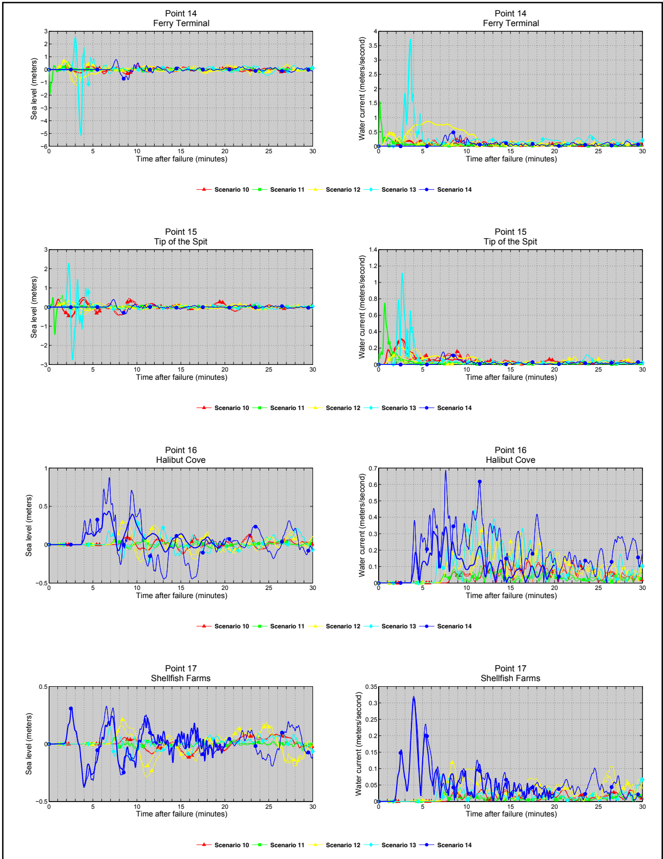
Figure A6, continued. Time series of water level (left column) and velocity (right column) for landslide scenarios 10-14 at selected locations shown in figures A1 and A2.
